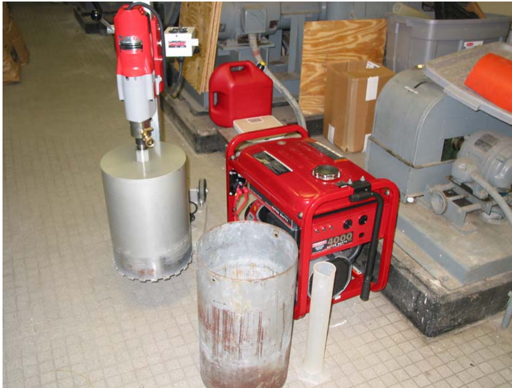
Figure 7: Coring Rig, Core Bit, Single-Ring Infiltrometer, and Generator
