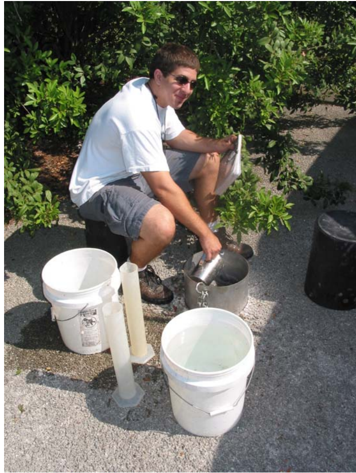
Figure 9: Pervious Concrete Pavement Core Test
