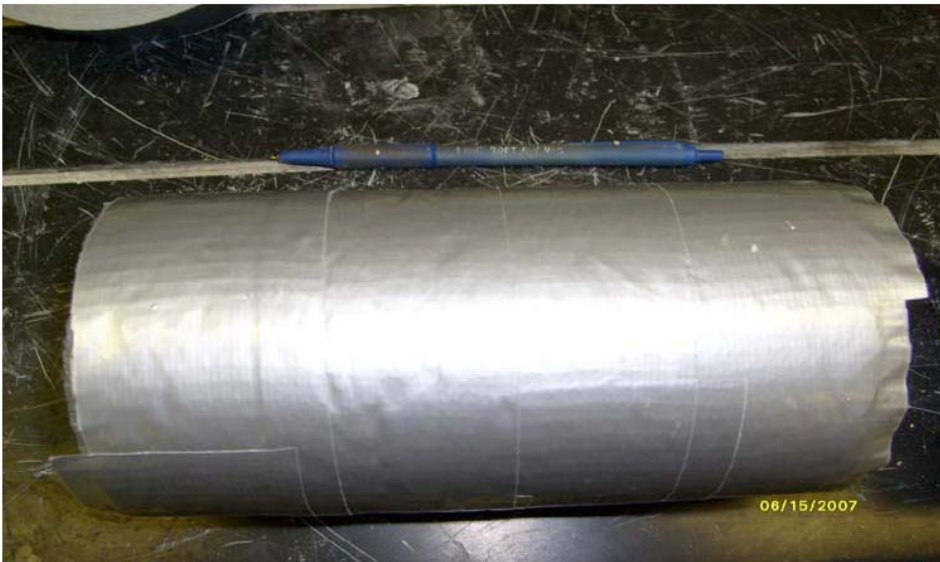
Figure 6: Sealed specimen for hydraulic conductivity testing
