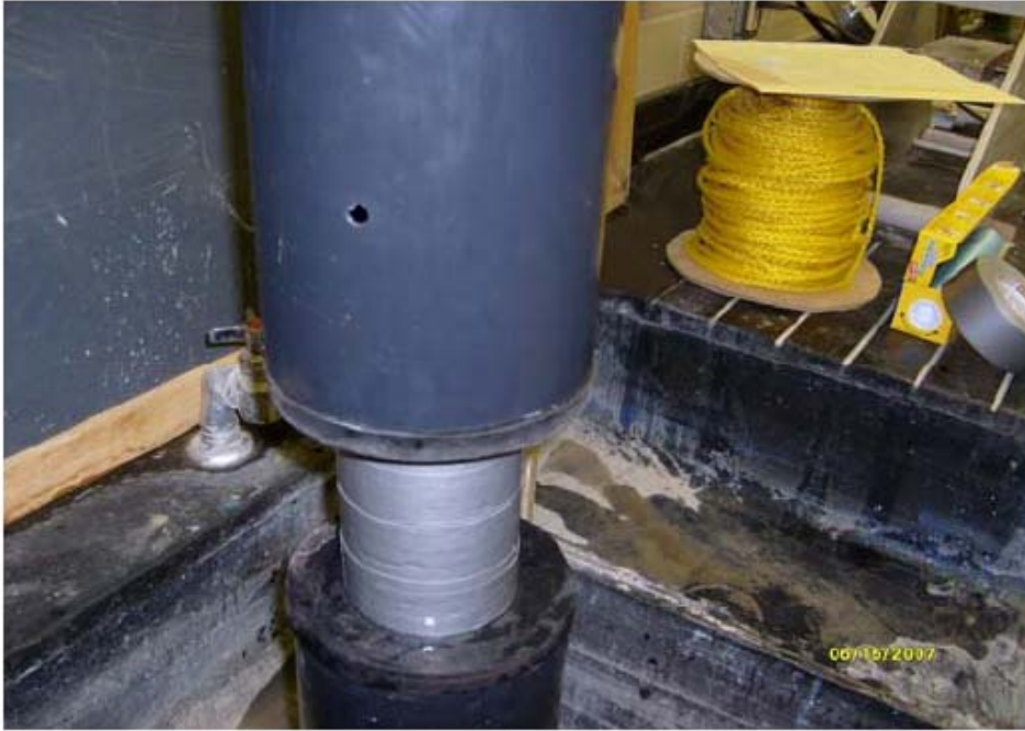
Figure 7: Laboratory hydraulic conductivity testing
