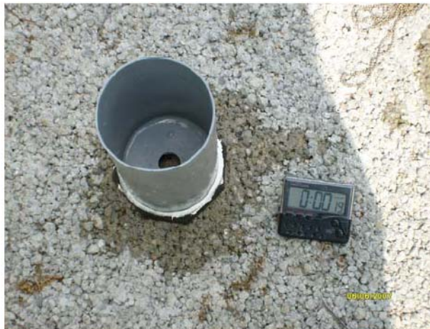
Figure 4: Drain time Apparatus
