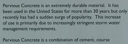
Pervious Concrete is a combination of cement, course aggregate and little or no sand. This mixture creates an open-cell pavement that allows rainwater to filter through to underlying soil. By imitating natural ground cover, Pervious Concrete is an excellent and durable choice for storm water management.
