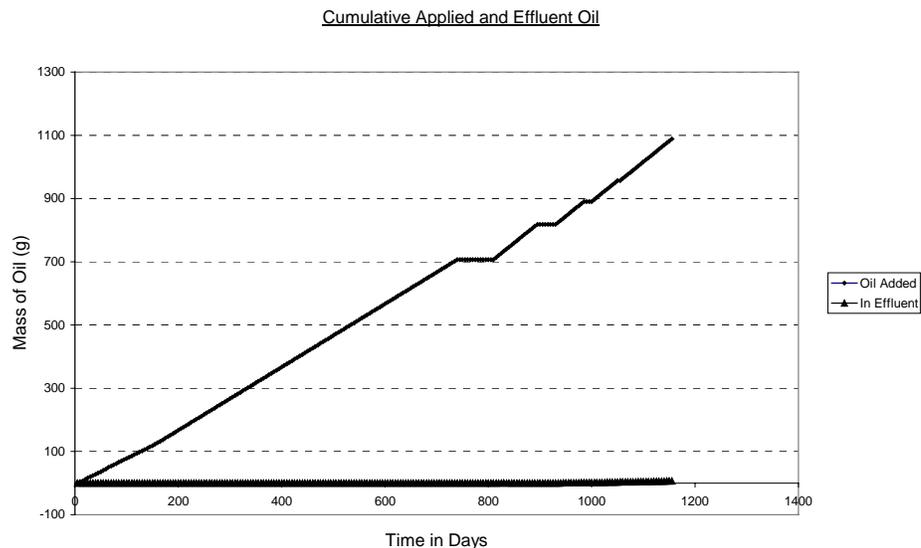
Fig 7 Graphs of cumulative mass of oil added (upper line) and released in effluent (lower line) For First 1150 days of experiment.
