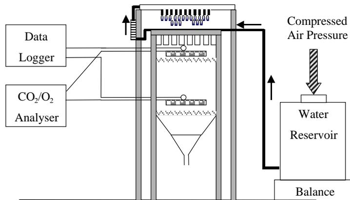
Figure 2. Rainfall simulation system and monitoring components.
