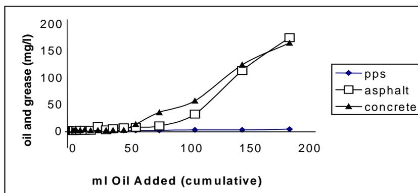
Fig 3 Graph of cumulative volume of oil added against concentration of oil released for PPS, asphalt and concrete (means of three replicates) Horizontal graph axis set at  $y = -5\text{mg/l}$  for clarity.
