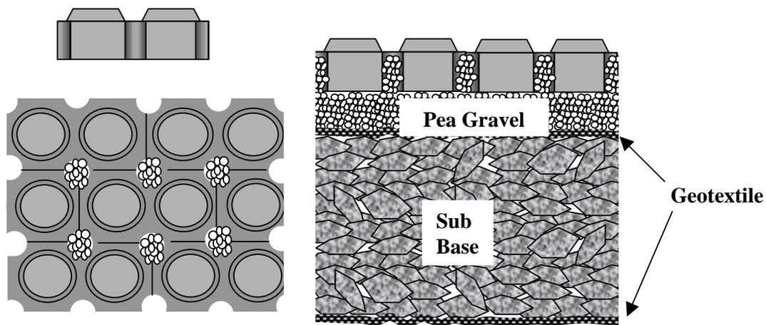
Figure 1 General arrangement of the porous parking surface
