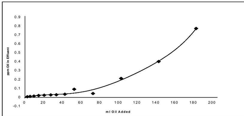
Fig 4 Graph of cumulative volume of oil added against concentration of oil released for PPS only
